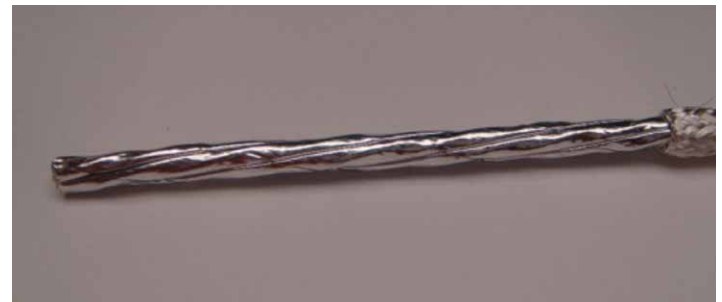
Figure 46: Exposing the foil
