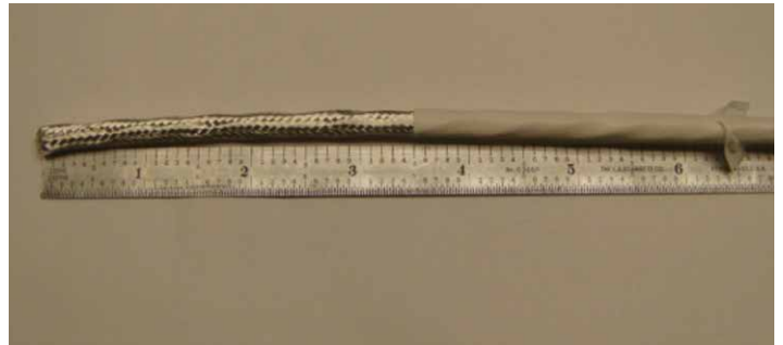
Figure 13: Exposing the braid
