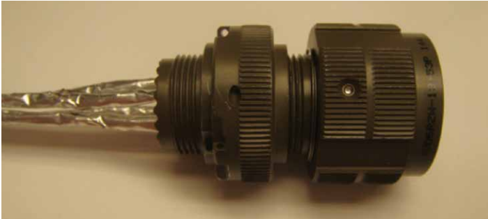
Figure 37: Connecting the grommet to the plug
