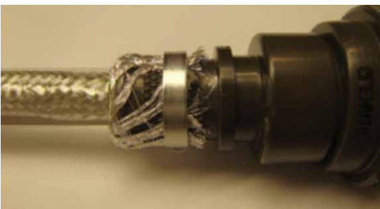
Figure 71: Attached Band-It® clamp
