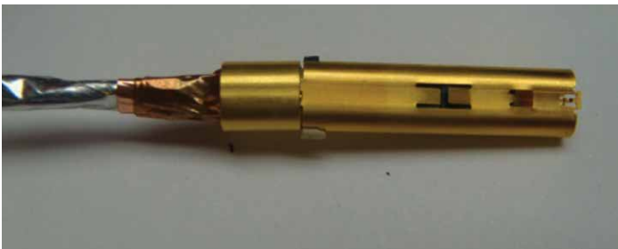
Figure 64: Positioning the ferrule
