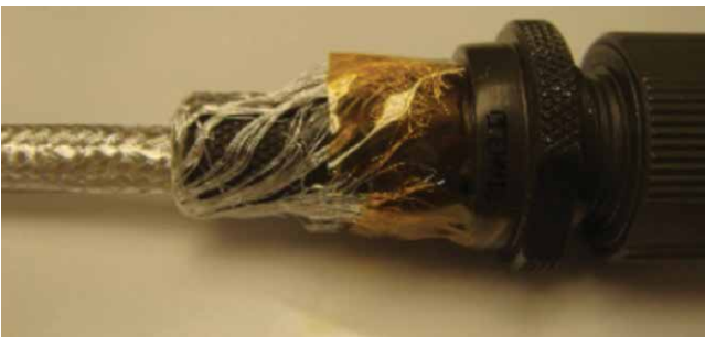
Figure 38: Returning braid to connector
