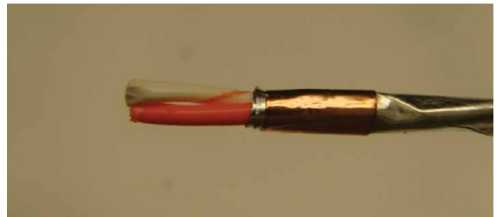
Figure 52: Removing polyimide tape and foil
