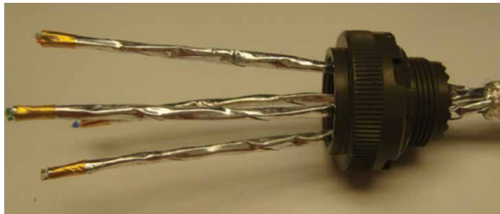
Figure 50: Positioning the grommet near the braid
