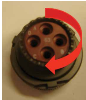
Figure 48: Inserting each pair into connector grommet
