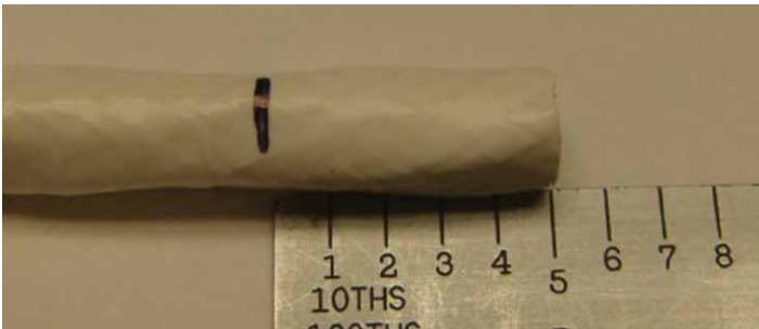
Figure 11: Marking the cable
