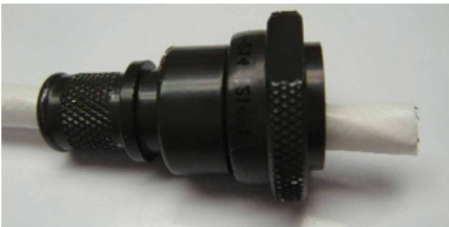
Figure 10: Inserting backshell on the cable
