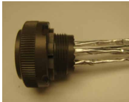
Figure 49: Pairs inserted in connector grommet
