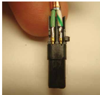
Figure 28: Attaching black rear insulator
