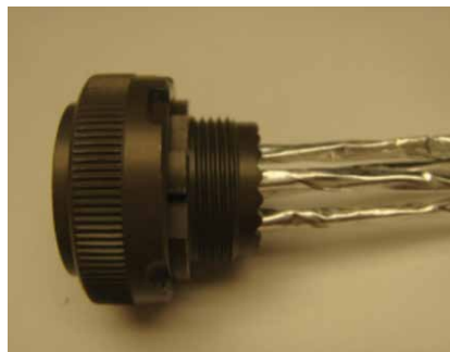
Figure 17: Pairs inserted in connector grommet
