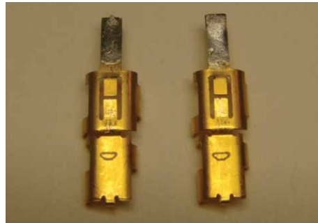
Figure 27: Tinning ears of outer body
