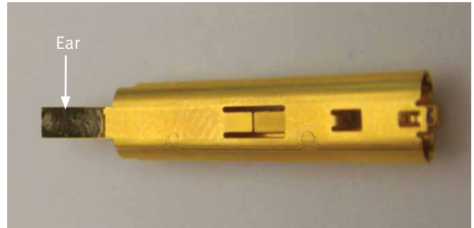
Figure 59: Tinning ears of outer body
