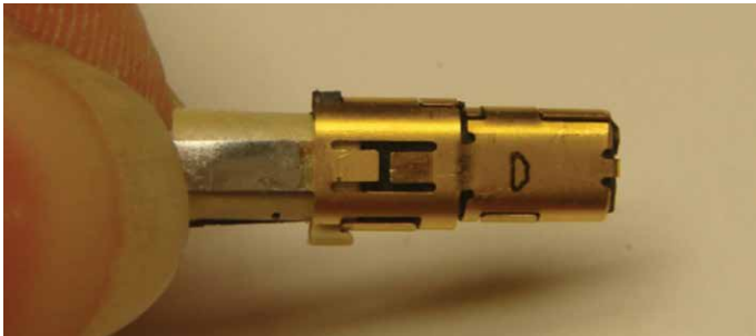
Figure 30: Locking outer body onto rear insulators
