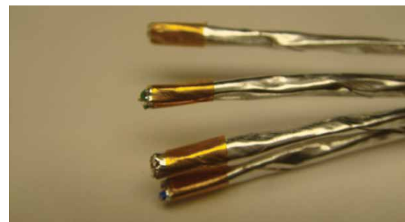
Figure 47: Taping each pair
