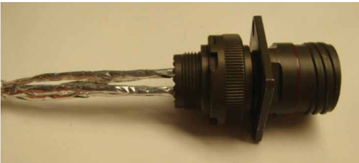
Figure 69: Connecting the grommet to the receptacle
