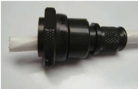
Figure 42: Inserting backshell on the cable
