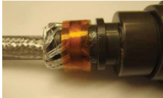
Figure 40: Wrapping Band-It® clamp
