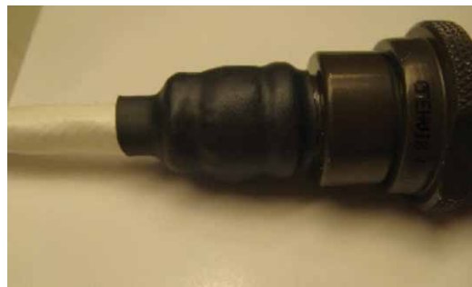
Figure 73: Shrinking tubing over backshell
