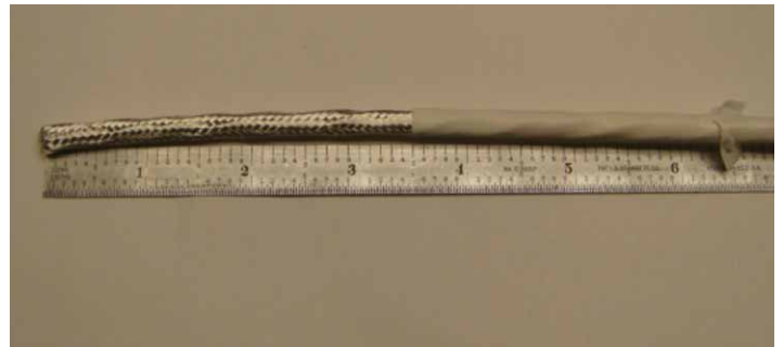
Figure 45: Exposing the braid
