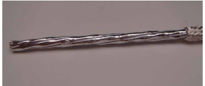
Figure 14: Exposing the foil
