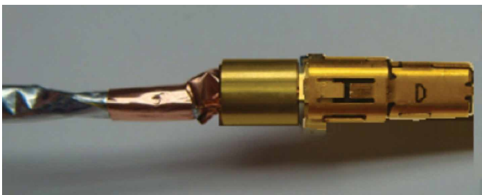
Figure 32: Positioning the ferrule
