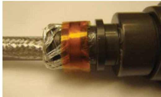
Figure 72: Wrapping Band-It® clamp
