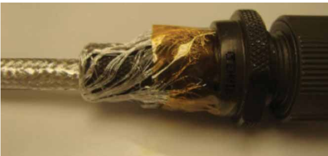
Figure 70: Returning braid to connector
