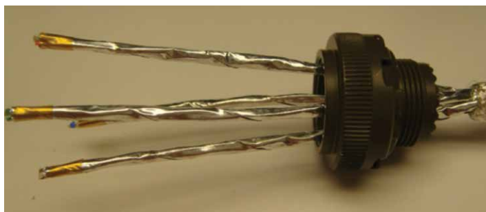
Figure 18: Positioning the grommet near the braid
