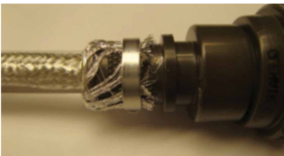
Figure 39: Attached Band-It® clamp
