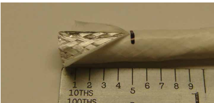
Figure 44: Slitting the cable jacket
