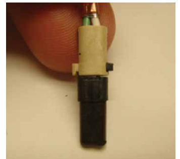
Figure 29: Attaching beige rear insulator
