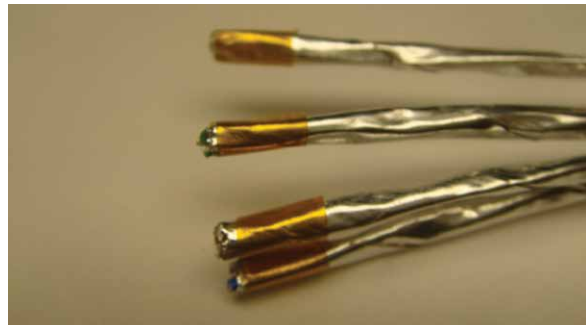
Figure 15: Taping each pair
