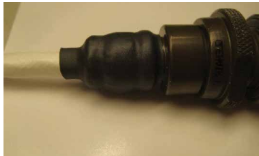
Figure 41: Shrinking tubing to backshell
