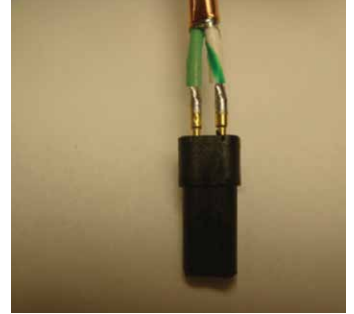
Figure 58: Soldering the twisted pair
