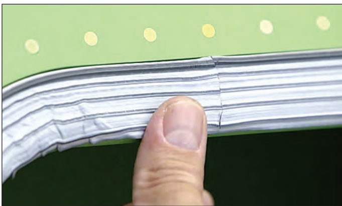
Figure 25: Adhering the two edges of the tape
