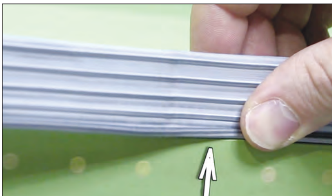
Figure 21: Positioning tape on panel edge
