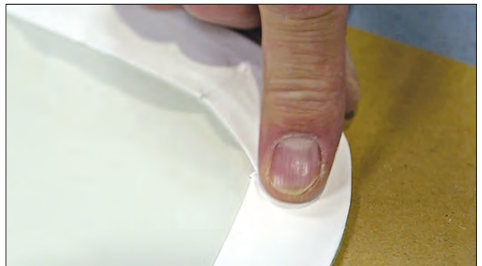
Figure 13: Sealing the tape around curve
