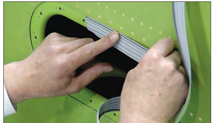
Figure 22: Positioning tape on frame
