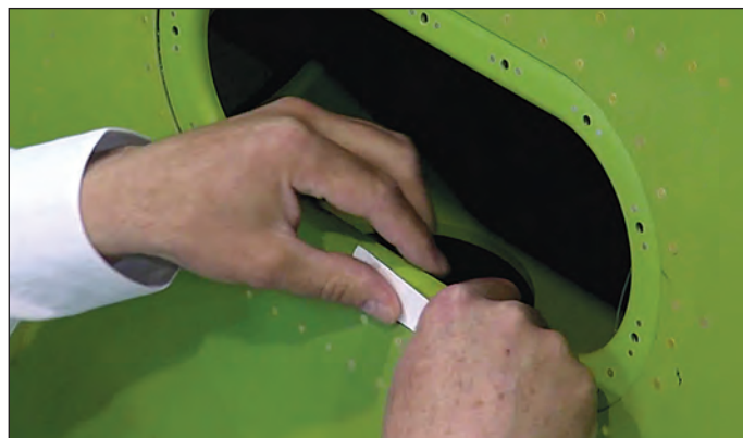
Figure 5: Positioning tape on frame
