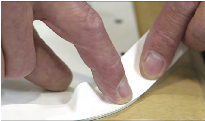
Figure 8: Forming a curve around panel
