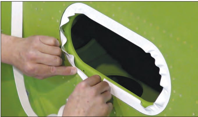
Figure 9: Forming a curve around frame
